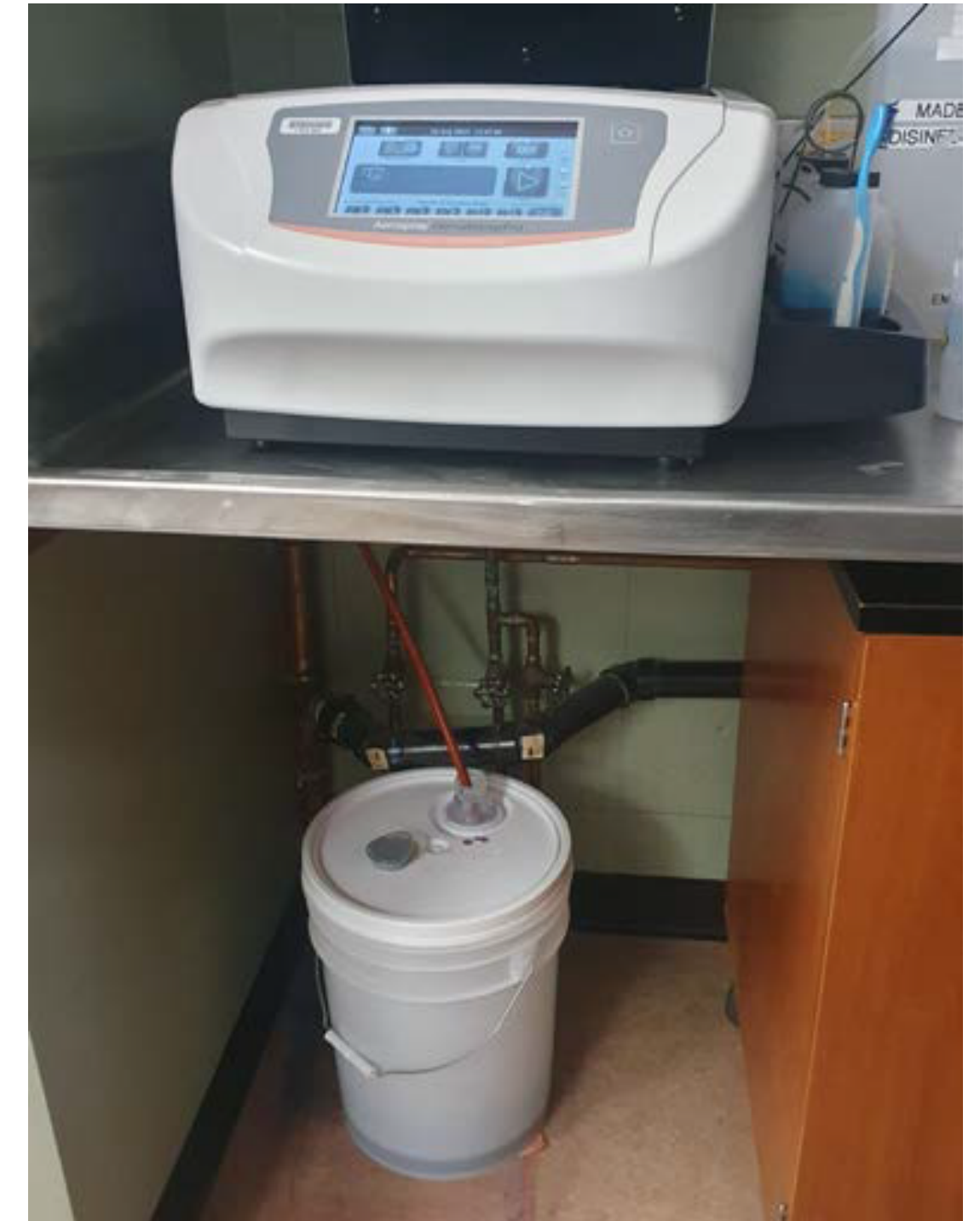
Figure 6: Slide stainer liquid waste collection system after two weeks worth of collection. Photo credit: Christine Henderson
